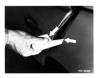
13 Check window frame in ranges A, B and C and straighten, if required.
