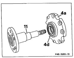
31 Insert drive shaft (11) with bearing flange cap (4a) into pump housing (2a). At the same time turn shaft carefully until the eccentric (arrow) of the drive shaft can be pushed into the bearing sleeve (5f).
