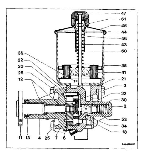
25 Insert filter set (41), spring (43) and plastic sleeve (60), compress slightly and install new self-locking nut (61). Fit on end cover (45), screw on breather cap (47).
