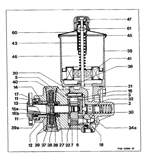
43 Insert filter set (41), spring (43) and plastic sleeve (60), compress slightly and install new self-locking nut (61). Fit on end cover (45), screw on breather cap.
