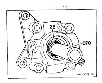
28 Press spacer ring (27) into the housing (4) with groove facing seal.
