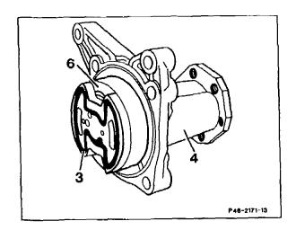
23 Insert O-rings in bearing flange, then insert bearing flange (4) in the pump housing and attach with the hexagon bolts (25).
