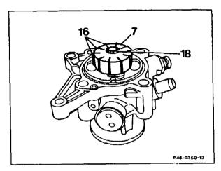
38 Insert vanes (10 off) into the rotor with the rounded metallic glossy sides (arrow) facing the cam insert.
