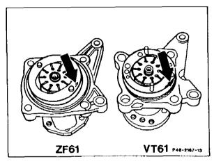
21 Insert vanes (10 off) into the rotor with the rounded, metallic glossy sides (arrow) facing the carn insert.
