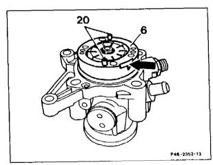
40 Fit pressure plate (3) with the ground face pointing toward cam insert (6). Fit O-rings (26b) onto the pressure plate with grease.
