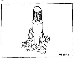
18 Insert drive shaft (11) into the bearing flange (4). After this, fit rotor (7) with the chamfer on the inner diameter facing the flange of the drive shaft.
