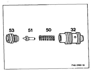
25 Check both sealing cones (high-pressure expansion hose, return pipe connection). Replace misshapen sealing cones. This is done by cutting a thread with M7 or M10 a few thread turns deep into the sealing cone. Withdraw the sealing cone from the housing with an M7 or M10 bolt.
