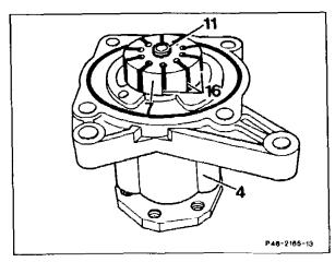
8 Remove drive shaft (11) from the bearing flange (4).
