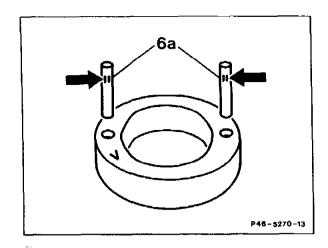
37 Insert cam insert (6) with direction of rotation arrow upwards on the bearing flange (4). At the same time the straight pins (6a) must be above the centering bores (arrow).
