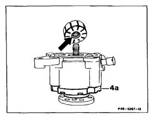
34 Mount new locking ring (11a). The locking ring must seat correctly in the groove (arrow) of the drive shaft.
