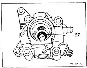
21 Pull out radial seal ring and washer (28) with internal extractor 000 589 33 33 00. Examine bronze bush in housing (4) for signs of damage and wear, replace housing, if necessary.
