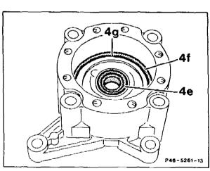
17 Withdraw radial seal ring (4e) with internal extractor 000 589 33 33 00. Check bronze bush in housing (4) for damage and wear, replace if required.
