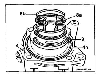
39 Insert bearing flange (4) in pump housing (2) and fasten with 4 bolts M8 (4b). Tightening torque 25 Nm.
