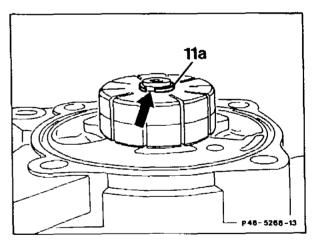
35 Insert vanes (7a, 10 vanes) in the rotor (7). Insert vanes with the rounded, metallic glossy sides towards the cam insert in the rotor.
