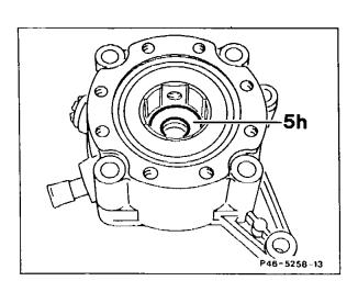
14 Tap bearing flange housing (4) between two blocks of wood until the piston support ring (5) can be removed.
