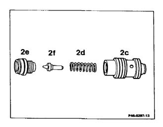
22 Insert compression spring (2j) and flow control valve (2c) in pump housing (2).
