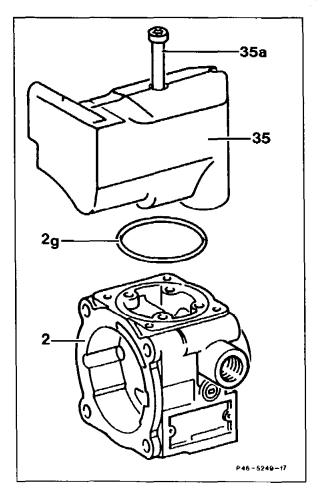
40 Insert O-ring (2g), mount reservoir (35) on pump housing and screw on with bolts (35a, 4 bolts).
