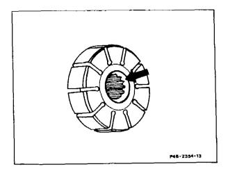
37 Install new locking ring (18). The locking ring (18) must be correctly seated in the groove of the drive shaft.
