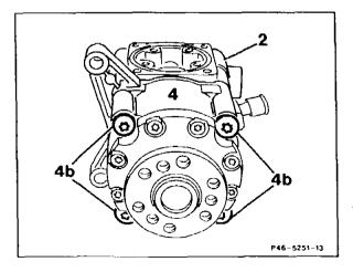
Note models 129.066/067, 140.04/050/051 Insert O-ring (2g) mount end cover (2k) and tighten with four bolts (arrow). Tightening torque: 8 Nm
