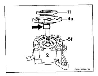
32 Fasten bearing flange cap (4a) with 8 screws M6 (4c).
