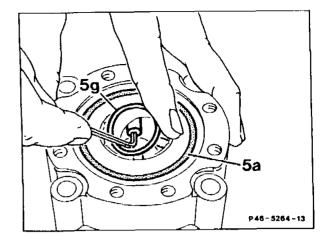
29 Insert bearing sleeve (5f) in bearing shell (5g).
