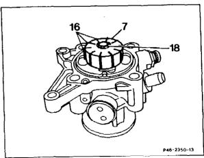
8 Detach rotor (7) from the drive shaft (11) with a plastic-headed hammer and take off together with the vanes (10 off). Check the vanes (16) in the grooves of the rotor (7); they must slide easily in the rotor.
