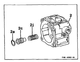
19 Clamp flow control valve (2c) in the vise at an unground section and unscrew the valve screw (2e) of the pressure relief valve.
