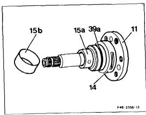
32 Carefully insert drive shaft (11) together with bearing flange (14) into the housing (do not damage seal). Ensure that the groove for the roll pin (19) is parallel to the roll pin bore. Knock roll pin (19) into the housing.
