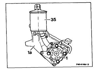
Loosen hose clamp, disconnect hose (arrow) and set aside. Unscrew bolts (46) and remove tandem pump (1) from support (1a).
