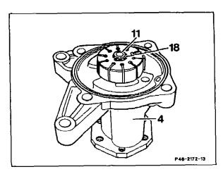
7 Detach rotor (7) with a plastic-headed hammer from the drive shaft (11) and take off together with the vanes (10 vanes). Examine the vanes (16) in the grooves of the rotor (7); they must slide easily in the rotor.
