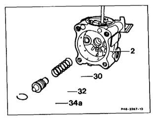
24 Clamp flow control valve (32) in a vise at a part which is not ground and unscrew valve screw (53) of the overpressure valve.
