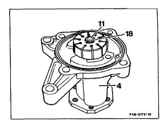
20 Insert the carn insert with the cast or stamped-in direction of rotation arrow (arrows) facing upwards into straight pins on the pump housing.
