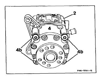
5 Remove O-ring (4h) in bearing flange (4), check, replace if required.
