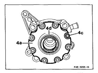
33 Push rotor onto the drive shaft so that the chamfer on the inside diameter (arrow) points towards bearing flange cap (4a).
