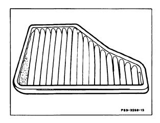
Dust filter for vehicles not equipped with active charcoal filter system
