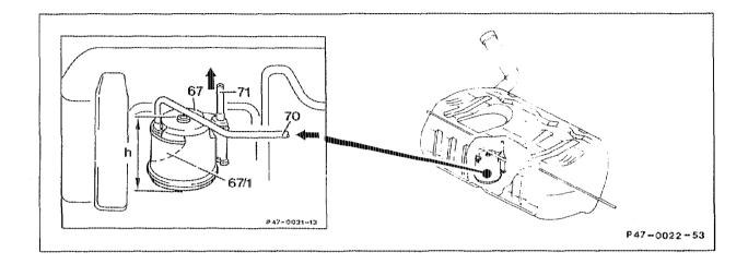
67 67/1 Splash bowl Separating chamber 70 71 Return pipe Riser pipe
