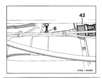
42 Vacuum element for right fresh air/recirculated air flap
