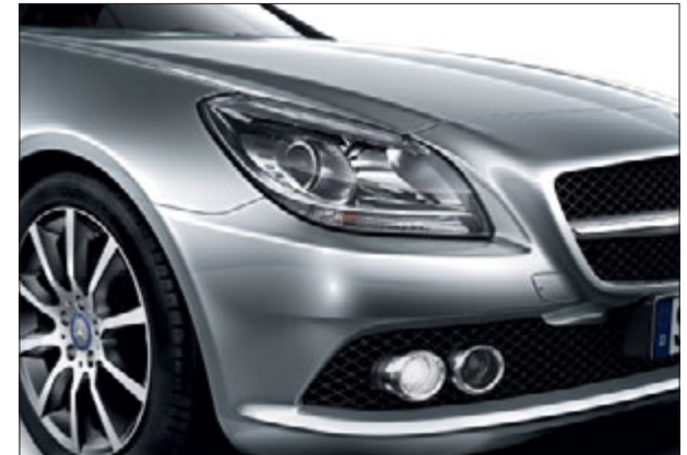
Clear-lens headlamps, daytime running lamps and front fog lamps
