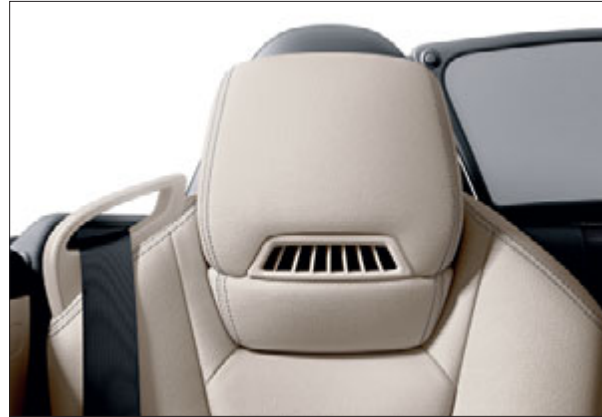
AIRSCARF neck-level heating
