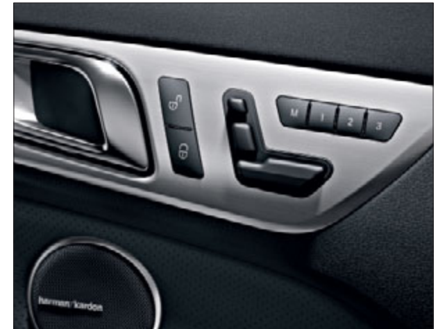
The electric seat adjustment with a memory function in the SLK
