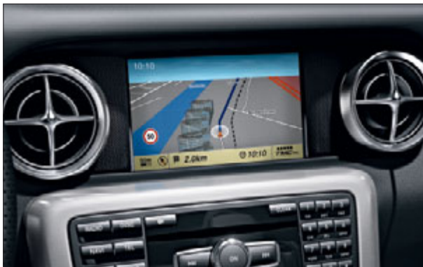
The information from the Speed Limit Assist is shown both in the instrument cluster and in the COMAND Online's central display
