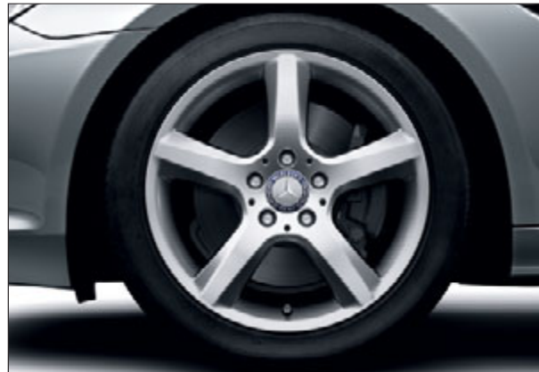
5-spoke light-alloy wheel with 225/45 R 17 front and 245/40 R 17 rear tyres (standard for SLK 250 BlueEFFICIENCY, Code 37R)
