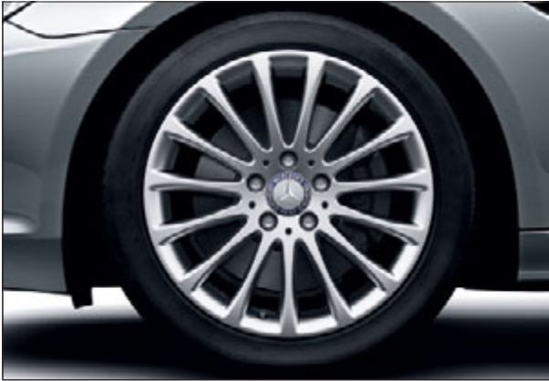
Multi-spoke light-alloy wheel with 225/45 R 17 front and 245/40 R 17 rear tyres (option, Code R81)
