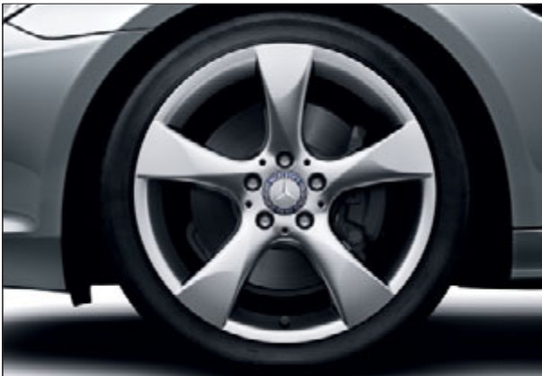
5-spoke light-alloy wheel with 225/40 R 18 front and 245/35 R 18 rear tyres (option, Code R32)
