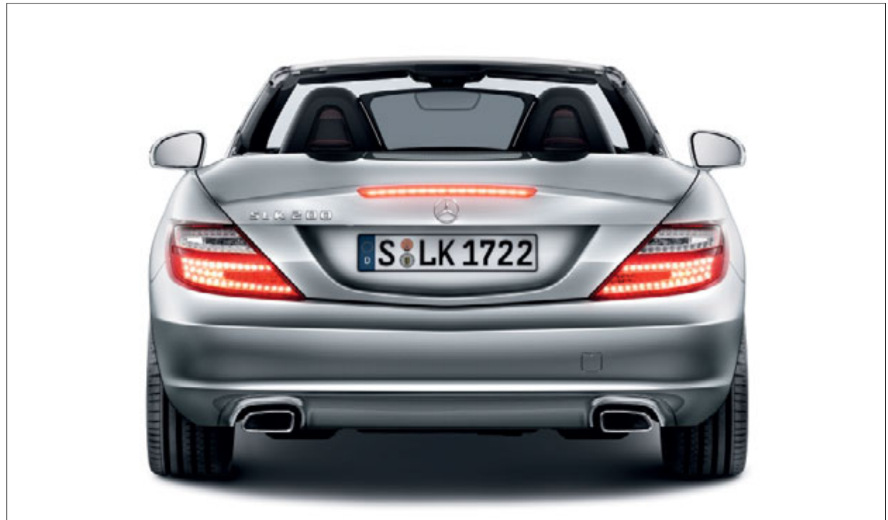
The adaptive brake lights contribute to perceptual safety by warning the traffic behind through flashing brake lamps as soon as the driver brakes heavily
