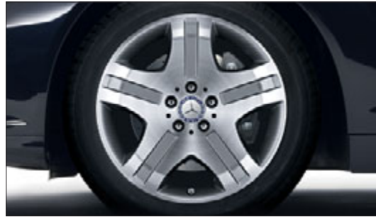
5-spoke light-alloy wheels with 255/45 R 18 front tyres and 275/45 R 18 rear tyres (standard for V12 engine)
