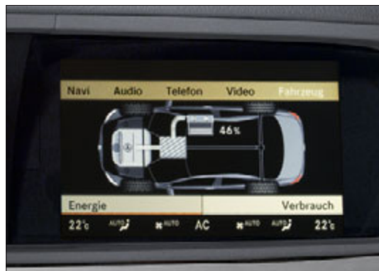
Energy flow display in the S 400 HYBRID model
