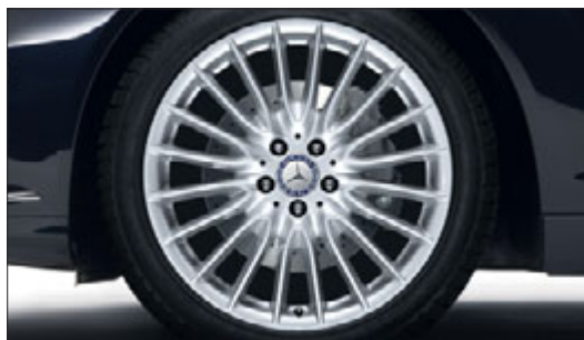
Multi-spoke light-alloy wheels with 255/40 R 19 front tyres and 275/40 R 19 rear tyres (optional extra)
