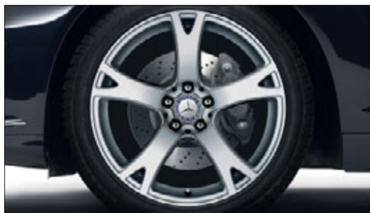
5-spoke light-alloy wheels with 255/40 R 19 front tyres and 275/40 R 19 rear tyres (optional extra)
