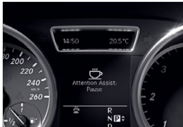
ATTENTION ASSIST can trigger a visual warning and an audible alarm
