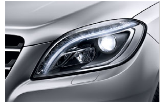
The Intelligent Light System with bi-xenon headlamps
