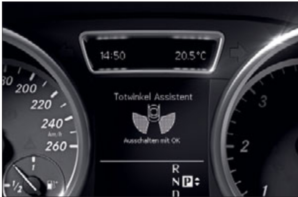
Active Blind Spot Assist is able to warn the driver about a vehicle in the blind spot
