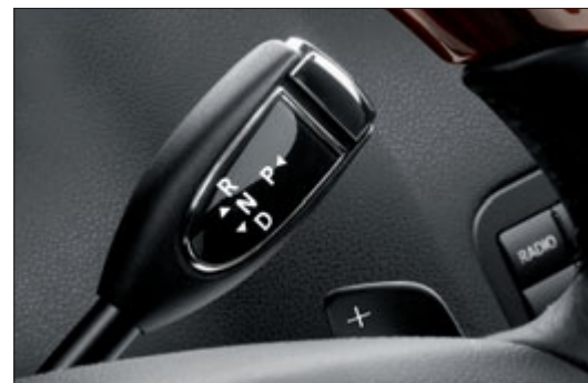
DIRECT SELECT steering-wheel shift paddles and selector lever
