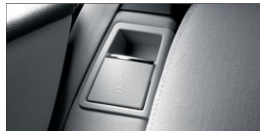
The release handle at the C-pillar makes it very easy to fold forward the rear seat backrest
