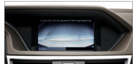
The reversing camera's wide-angle lens films the area directly around the rear of the car
