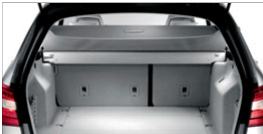
The EASY-PACK load compartment cover moves upwards when the tailgate is opened
