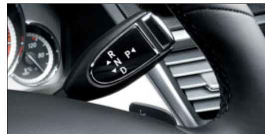
Fingertip transmission control with the DIRECT SELECT lever on the steering wheel
