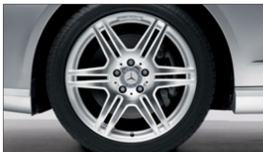
6-twin-spoke AMG light-alloy wheels with 245/40 R 18 front and 265/35 R 18 rear tyres, 245/40 R 18 front and rear tyres for 4MATIC (standard for AMG Sports package)
