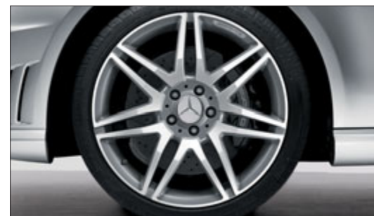
7-twin-spoke AMG light-alloy wheels with 245/35 R 19 front and 275/30 R 19 rear tyres, painted sterling silver (optional extra, Code 770)
