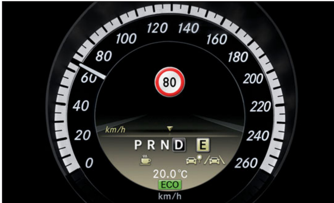
Speed Limit Assist can even indicate temporary speed limits
