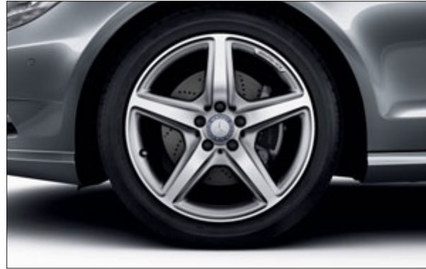
5-spoke AMG light-alloy wheels with 255/40 R 18 front and 285/35 R 18 rear tyres, painted titanium silver with a high-sheen finish (standard for AMG Sports package, Code 790)
