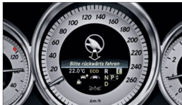
The display in the instrument cluster gives you a clear picture of the parking manoeuvres at all times
