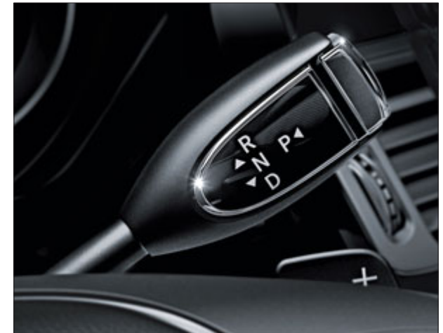
Transmission control with the DIRECT SELECT lever on the steering wheel
