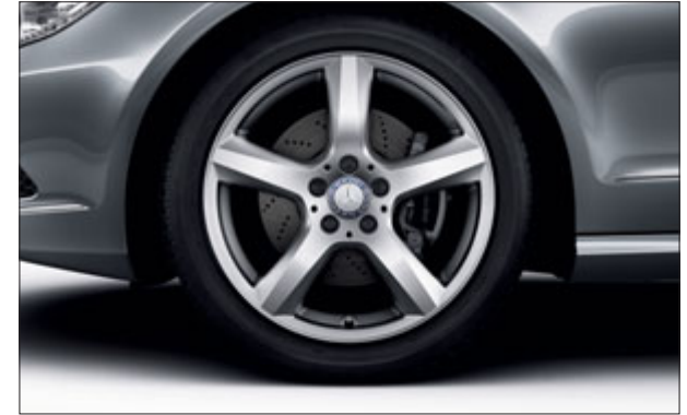
5-spoke light-alloy wheels in silver with 255/40 R 18 front and 285/35 R 18 rear tyres (standard for Exterior Sports package, Code R32, in anthracite Code R36)
