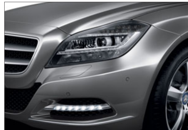
LED high-performance headlamps with LED daytime running lamps
