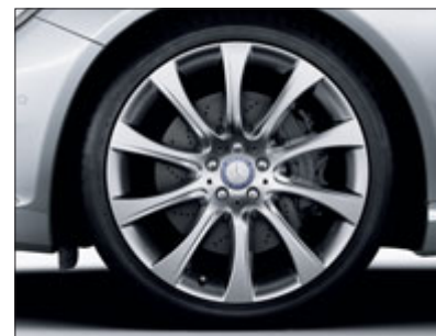
10-spoke "Alaraph" light-alloy wheels with 255/35 R 20 front and 275/35 R 20 rear tyres, 255/35 R 20 tyres all round on 4MATIC models, sterling silver (ex-factory accessories)
