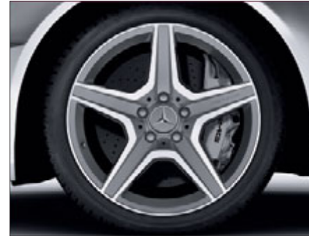
5-spoke AMG light-alloy wheels with 235/40 R 18 front tyres and 255/35 R 18 rear tyres, painted titanium grey with high-sheen finish (optional for C 63 AMG, Code 790)
