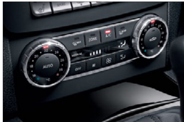
THERMATIC operates on the basis of sensor information including data for interior and exterior temperature as well as air humidity
