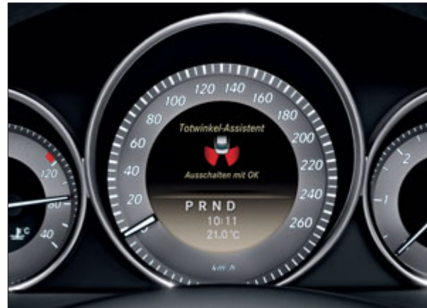
Blind Spot Assist can monitor the hidden-from-view areas alongside and behind the car in order to help the driver change lanes safely
