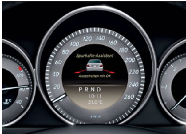
Lane Keeping Assist can make the steering wheel vibrate if the vehicle drifts unintentionally across lane markings
