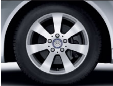
7-spoke light-alloy wheels with 195/60 R 16 tyres (Saloon, standard for C 180 CDI BlueEFFICIENCY, C 200 CDI BlueEFFICIENCY, C 180 BlueEFFICIENCY, Code R20)
