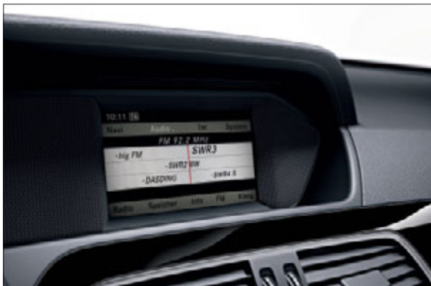
A Bluetooth® interface with hands-free system and the Audio 20 system with telephone keypad facilitate mobile communication
