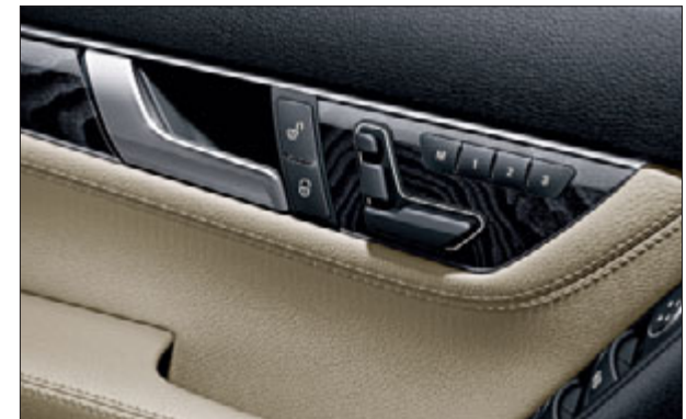
The ergonomic driver's seat moves into the pre-programmed desired position at the touch of a button
