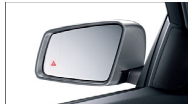
Blind Spot Assist is available as part of the optional Lane Tracking package
