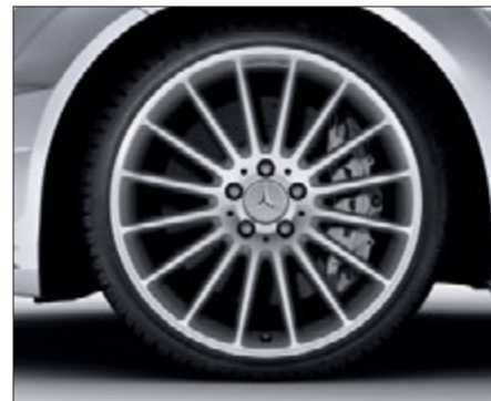
Multi-spoke AMG light-alloy wheels, painted titanium grey with a high-sheen finish, with 235/35 R 19 front tyres and 255/30 R 19 rear tyres (optional for C 63 AMG, Code 788)
