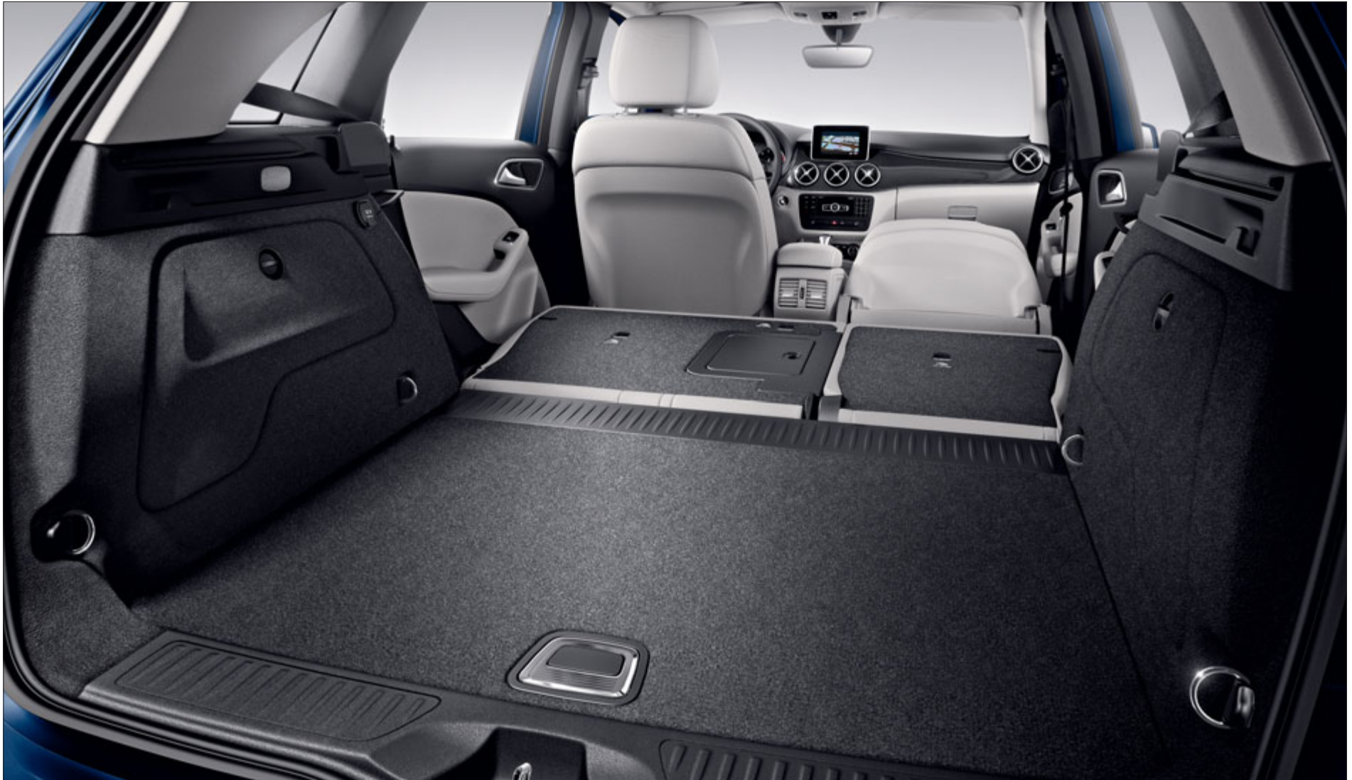
Fully folding down the rear seats allows a load compartment capacity of 1545 litres with a practically flat load bay
