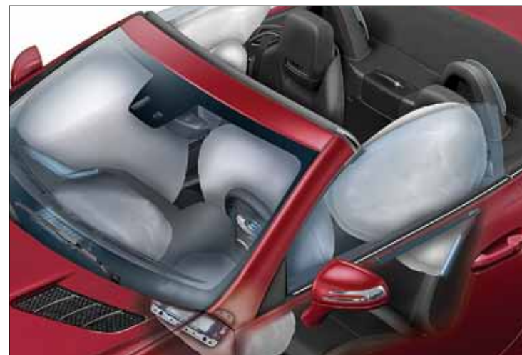
Head airbags reduce the risk of injury by providing additional support in the event of a collision 1,4 .
