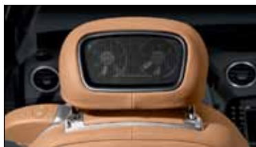
The AIRSCARF system.
