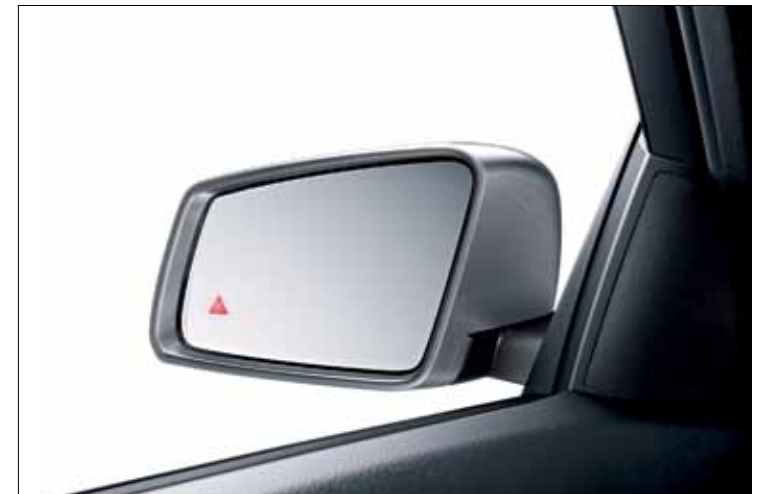
Blind Spot Assist alerts the driver if it identifies a risk of a collision while the vehicle is changing lanes.
