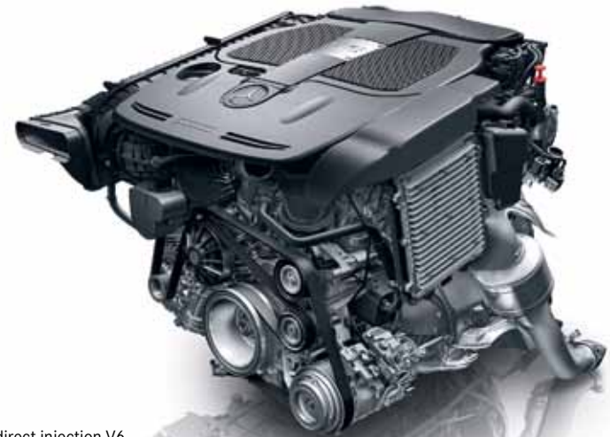
3.5 L direct injection V6.
