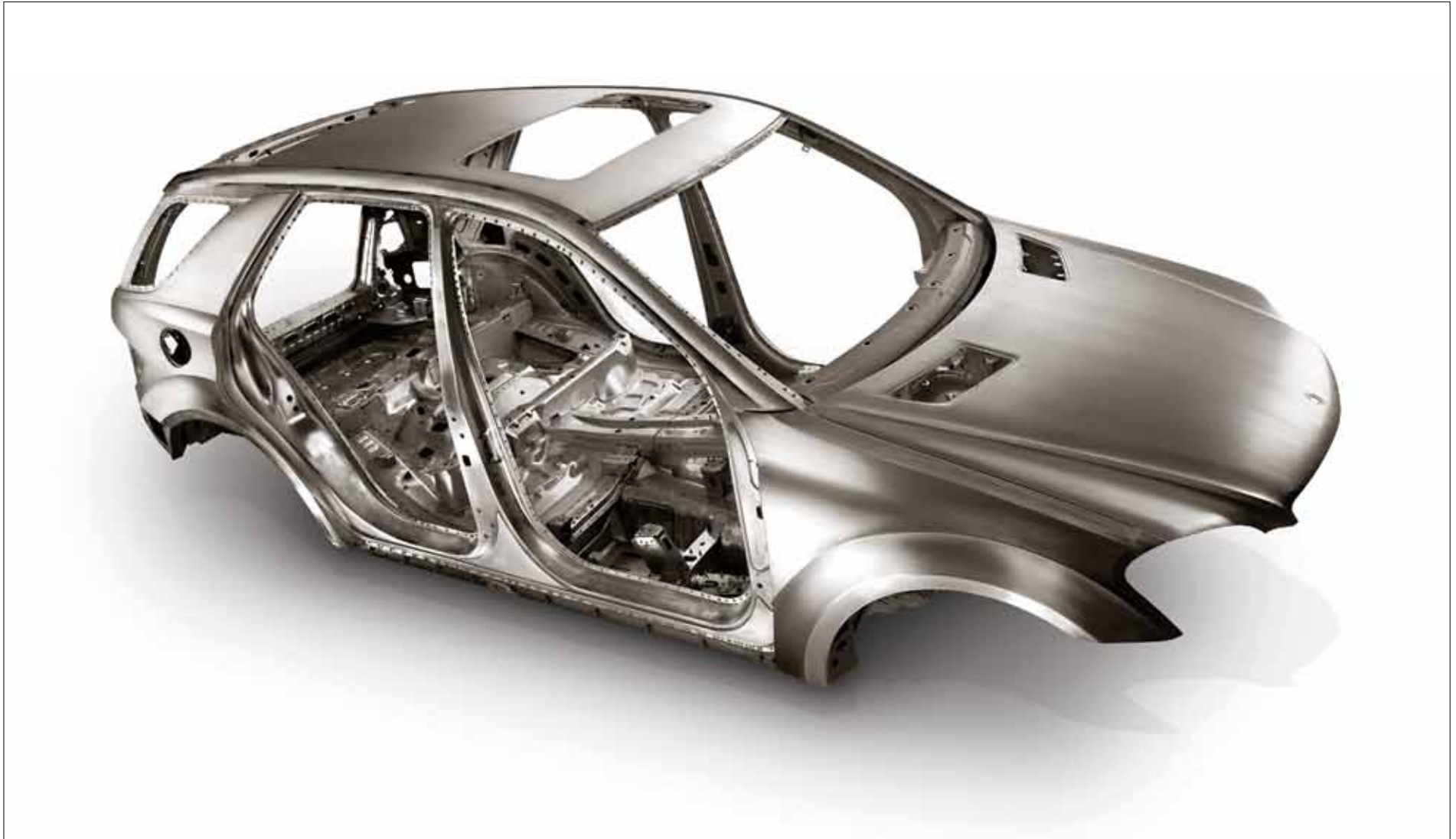
The energy-absorbing crumple zones in the front and rear sections, an extremely robust safety passenger cell, and the doors with special reinforcing elements form an effective defensive barrier in an emergency.
