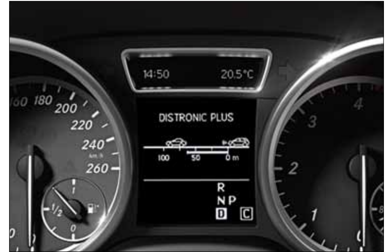
DISTRONIC PLUS reduces the chance of rear end collisions by automatically braking in the event of danger.
