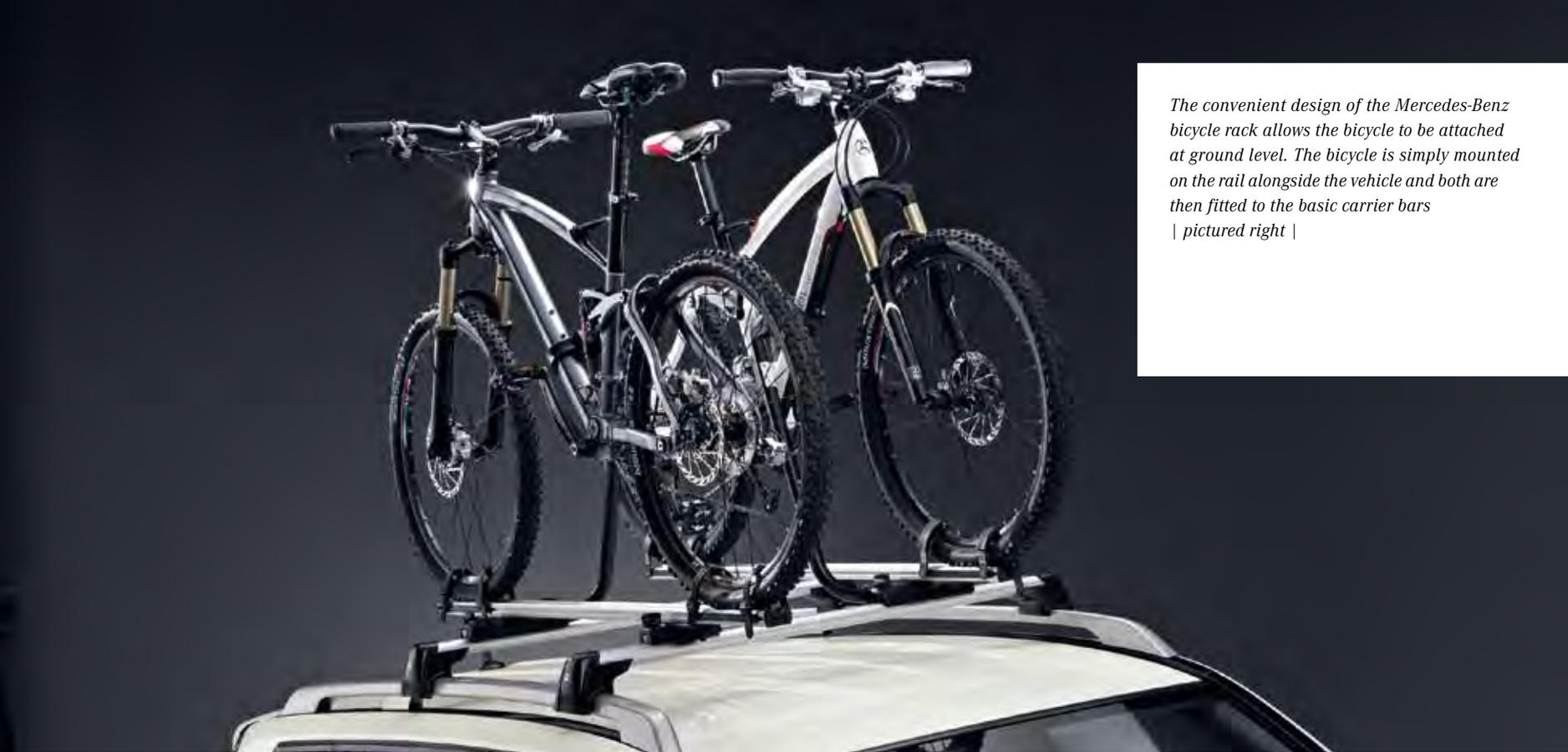
*The convenient design of the Mercedes-Benz bicycle rack allows the bicycle to be attached at ground level. The bicycle is simply mounted on the rail alongside the vehicle and both are then fitted to the basic carrier bars | pictured right |*
