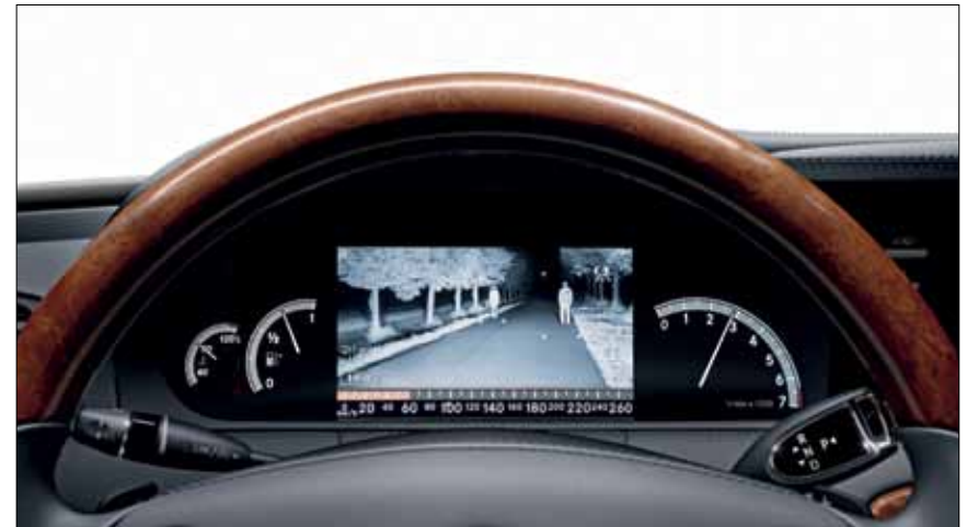
Night View Assist utilizes radar technology to assist during night time driving.
