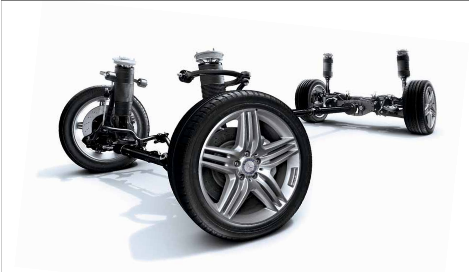
The Adaptive Damping System (ADS) allows for quick adjustments of the suspension to accommodate driving style.
