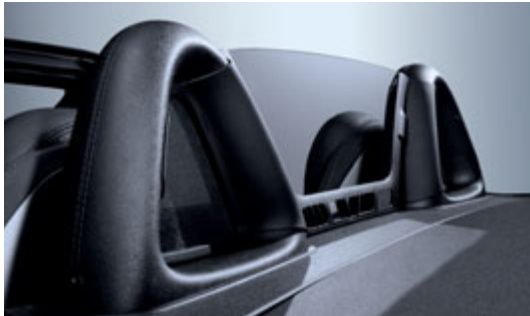
The perspex draught-stop reduces airflow turbulence
