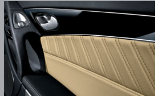
Trim in designo black piano lacquer (W69) and door centre panel with characteristic piping look in designo pastel yellow leather (X12)
