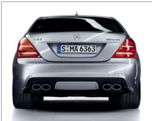
AMG sports exhaust system with chromed twin tailpipes
