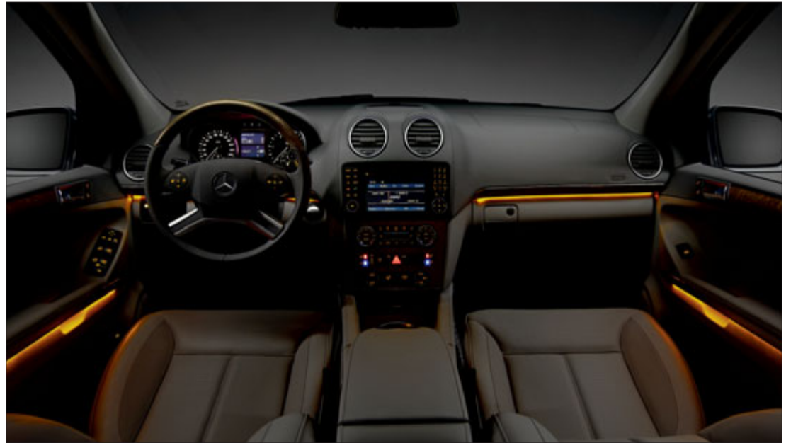
The ambient lighting lights up as a narrow band of LEDs along the wood trim strips, the dashboard and all four doors. Five levels of brightness can be selected via the menu in the instrument cluster
