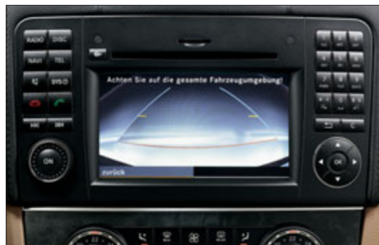
The reversing camera films the area around the tail end of the car
