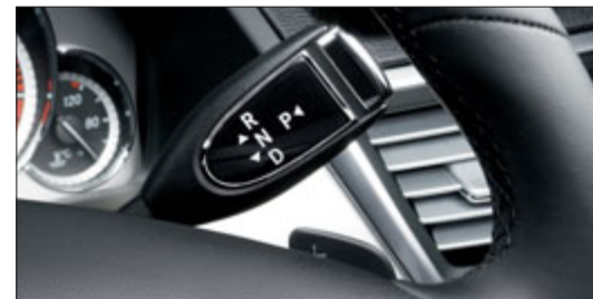
Transmission for the V6 and V8 engine variants operated at the push of a button using the DIRECT SELECT lever on the steering wheel
