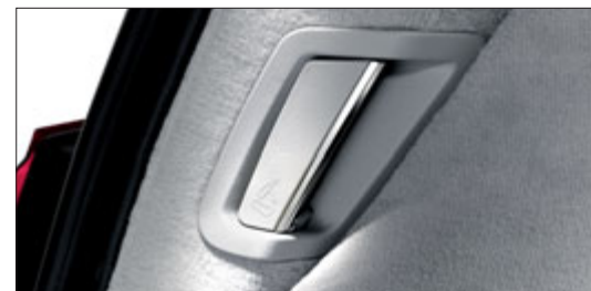
EASY-PACK quickfold at the D-pillar allows the rear seat backrest to be folded down, even from the boot
