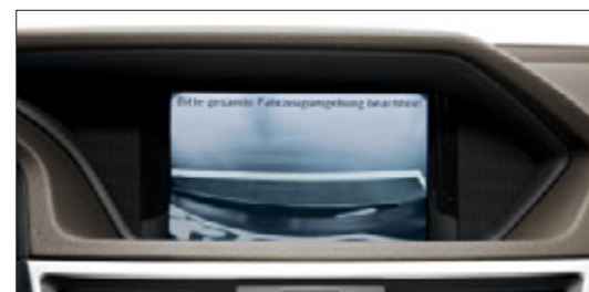
The reversing camera's wide-angle lens films the area directly around the rear of the car
