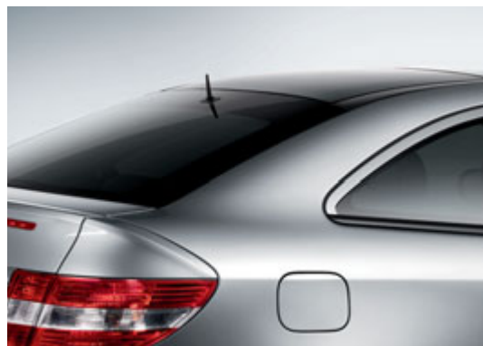
The heat-insulating dark-tinted glass at the rear
