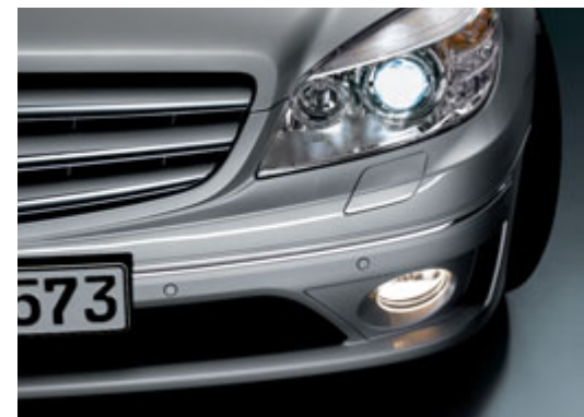
The bi-xenon headlamps with a cornering light function
