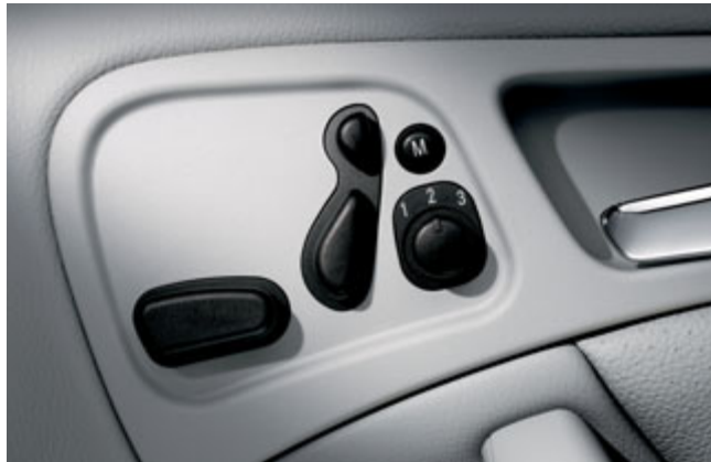
The electric seat adjustment with memory function
