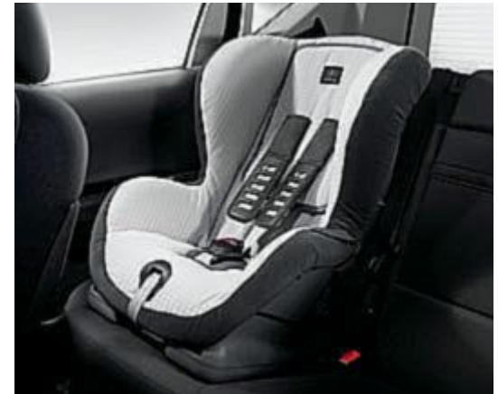
ISOFIX child seat attachment points in the rear with TopTether provide the best possible level of protection for your child, allowing a rigid connection between child seat and vehicle body
