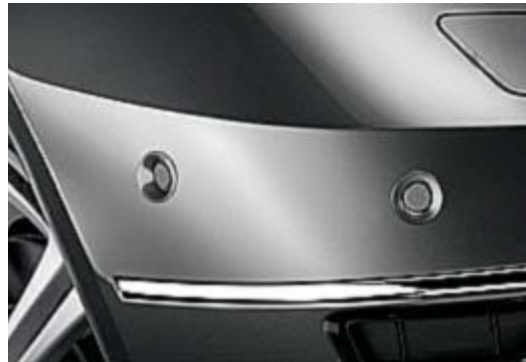
The distance sensors in the front and rear bumper monitor the parking process
