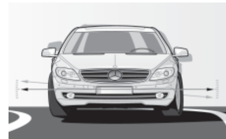
The ride height can be adjusted manually via the COMAND system for snowdrifts, low bottom clearance or rutted roads.
