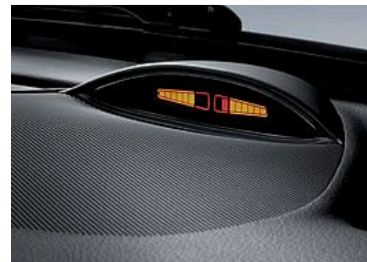
The PARKTRONIC system with LED display
