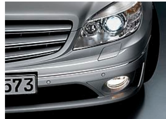
Bi-xenon headlamp and fog lamp/cornering light function
