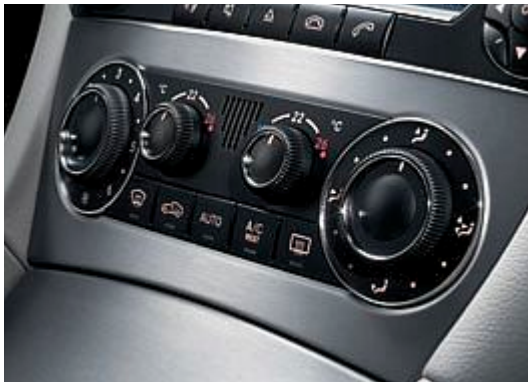
The automatic climate control with aluminium trim elements
