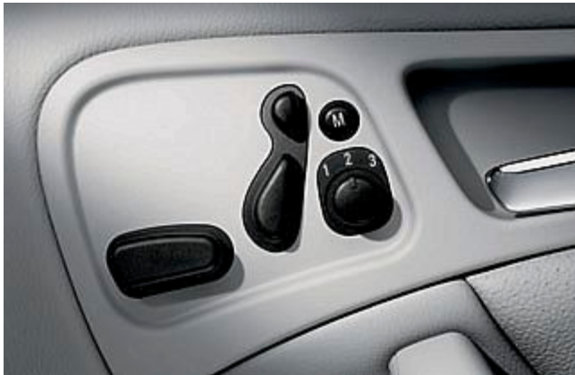
Electric seat adjustment with memory function
