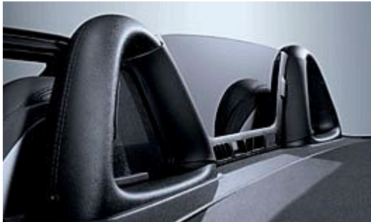
The perspex draught-stop reduces airflow turbulence
