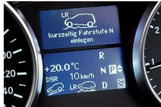
The off-road display in the instrument cluster
