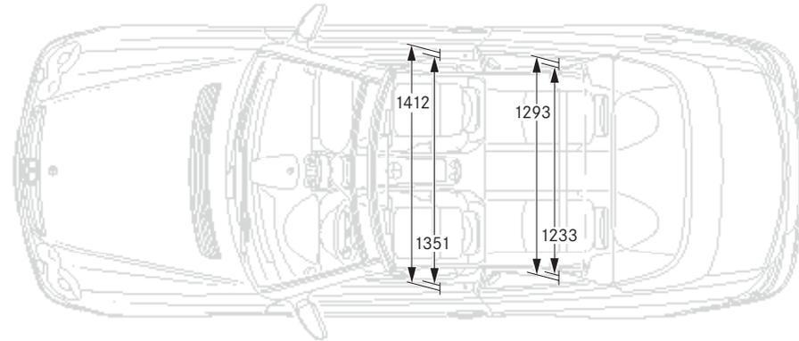
The dimensions shown are mean values (in mm) and apply to standard-specification vehicles carrying two occupants weighing 68 kg each
