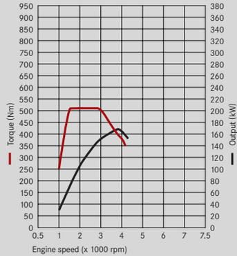
\* The torque curve shown is obtained in combination with 7G-TRONIC which is available as an option
