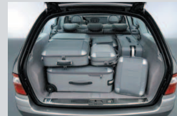
Load securing by nesting
