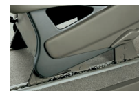
The seats in the Viano can be adjusted easily in increments of 25 mm
