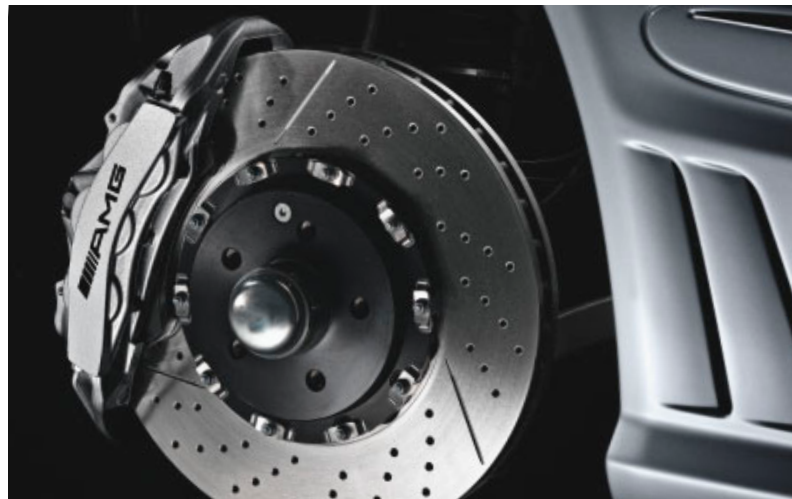
AMG braking system with composite brake discs
