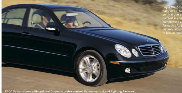
Enjoy the best of both worlds with the balanced ride of Airmatic Dual Control semi-active air suspension. Incredible comfort is yours as you ride on a cushion of compressed air. But corner aggressively, and Airmatic's Adaptive Damping System reacts instantaneously, firming up the suspension to reduce body roll and maximize control.
