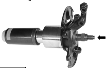
Wheel bearing extraction with KL-0040-61 A
