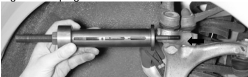
Fig. 4: Clamping bolt is extracted.
