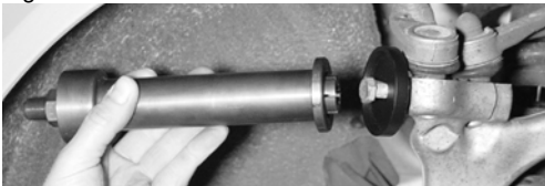
Fig. 4: Clamping bolt is extracted.
