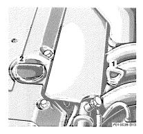
To check the engine oil level, park vehicle on level ground, with engine at normal operational temperature.
