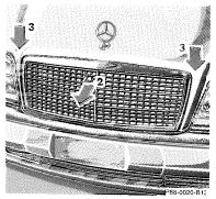
Pull handle (2) completely out of radiator grill and open hood (do not pull up or handle).
