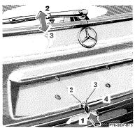
When the rear door and tailgate lock buttons are down, the rear doors and the tailgate cannot be opened from the outside or the inside, unless the door lock buttons are first pulled up.
