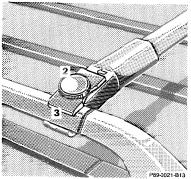
4. Turn clamping plates back (3) over roof railings and tighten the knurled-head screws (2).
