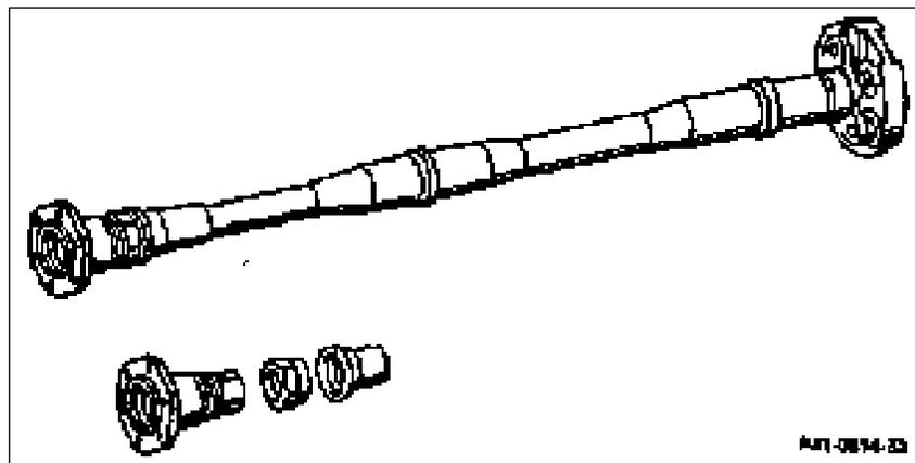
The propeller shaft connects the transfer case to the front axle differential.
