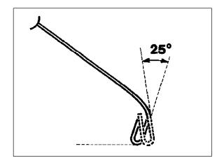
2.6 Allow front fender flare to curve smoothly back towards original, unflared line within the marked area (B).
