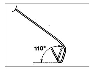
2.4 In the marked area (A), the fender flange is flattened down up to the inside of the fender in several stages. A plastic hammer must be used to avoid damaging the paint.
