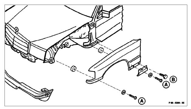
1.4 Press the side part of the bumper downwards and loosen and unscrew the bolts for fender fixing (A and B). Clamp a spacer between fender and body on the left and the right. The bore holes must align to permit troublefree fixing.
