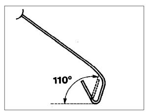
2.4 In the marked area (A), the fender flange is flattened down up to the inside of the fender in several stages. A plastic hammer must be used to avoid damaging the paint.
